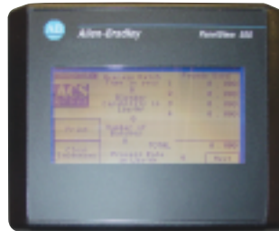
Real time display of process rate and material usage of each ingredient
